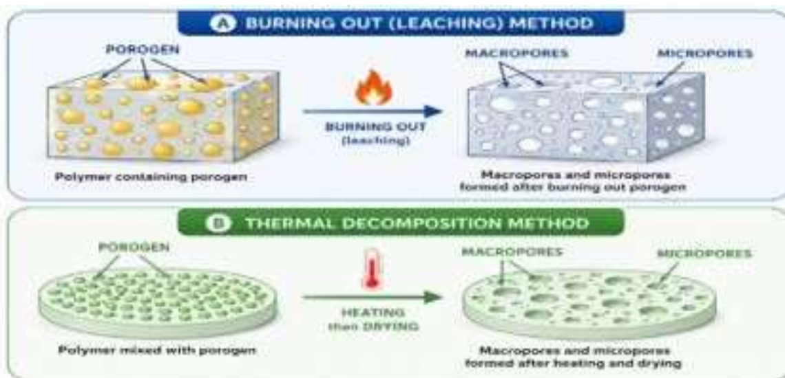
Figure 4: Microsphere preparation by porogen addition
